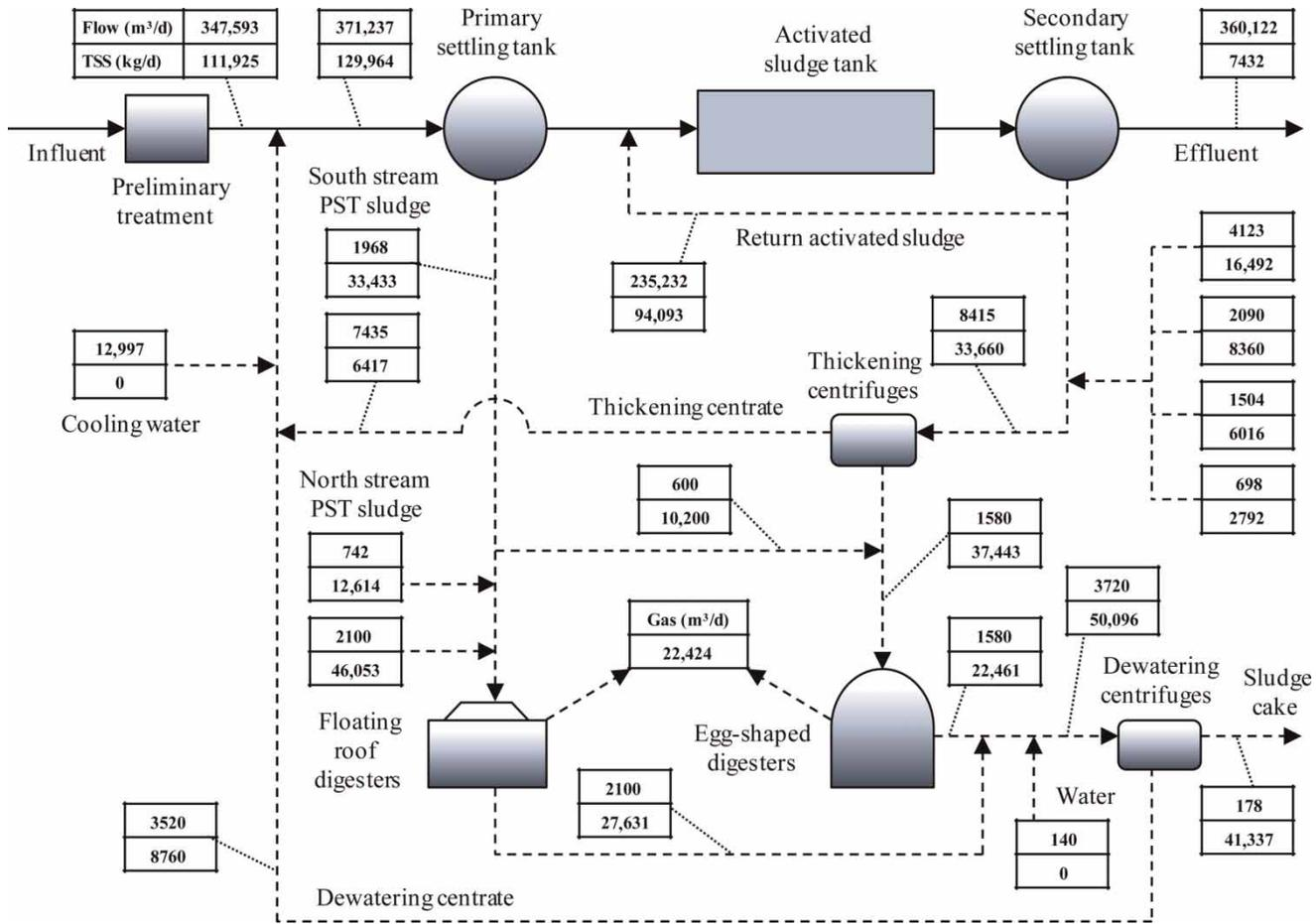
Figure 1 | Schematic layout of the hydraulic and solids flow in UluPandan WRP.
