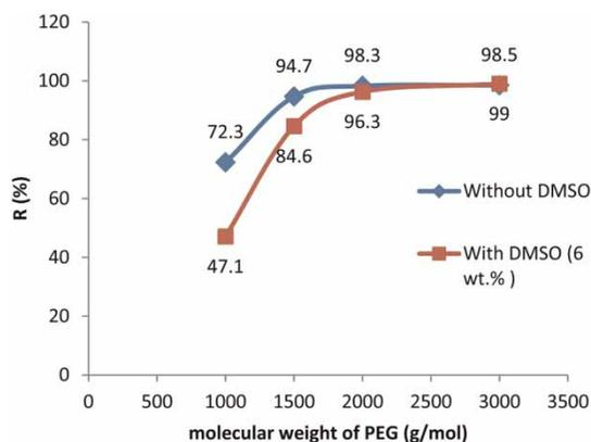
Figure 6 | Rejection of different molecular weights PEG.
