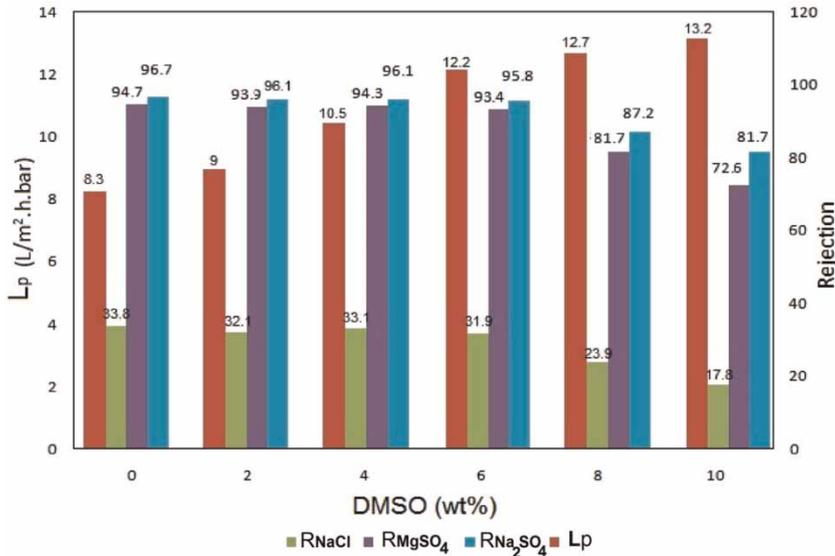
**Figure 4** | Effect of DMSO additive content on pure water flux and rejection; concentration of 2,000 ppm NaCl, Na<sub>2</sub>SO<sub>4</sub>, and MgSO<sub>4</sub>; operating pressure of 3 bar.
