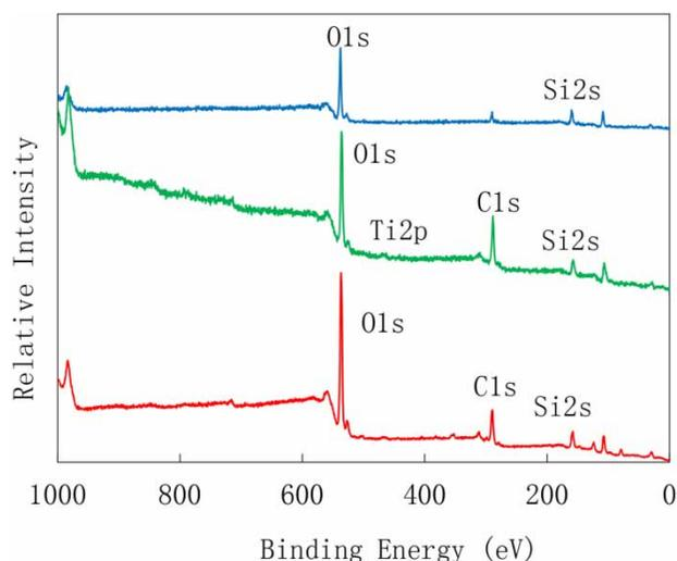
Figure 8 | XPS spectra of (a) UQS, (b) MQD-Ti and (c) MQD-Si.
