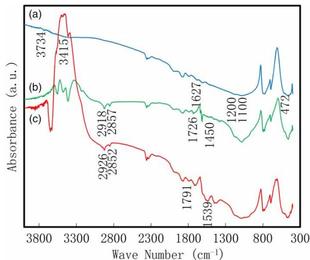
Figure 7 | FTIR spectra of (a) UQS, (b) MQD-Ti and (c) MQD-Si.
