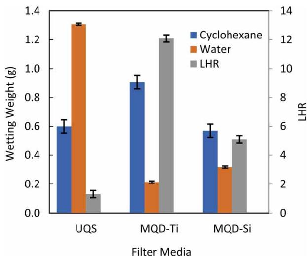
**Figure 2** | Cyclohexane and water wetting weights and LHR values of three samples.
