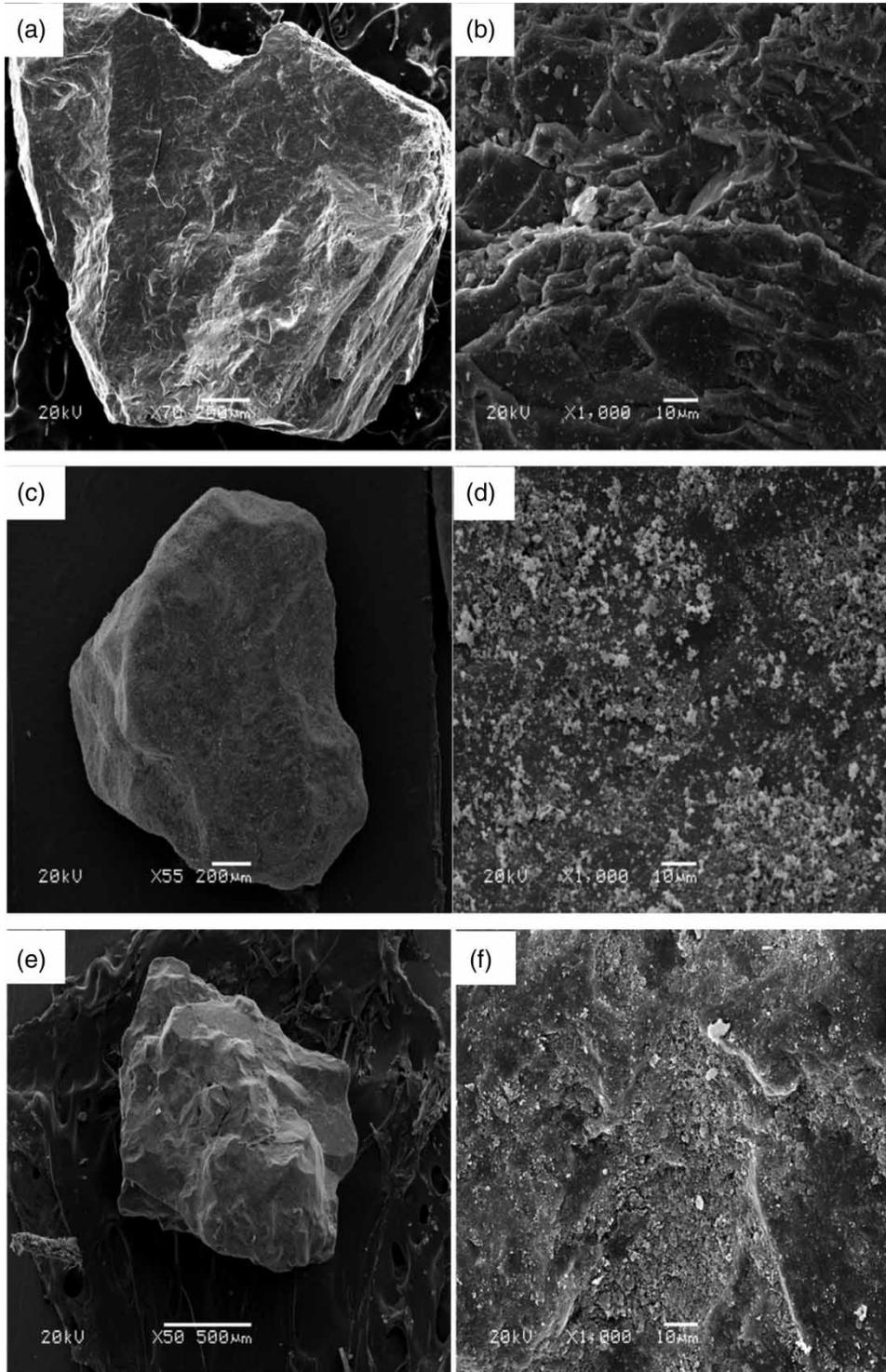
**Figure 6** | SEM micrographs of (a) and (b) UQS, (c) and (d) MQD-Ti and (e) and (f) MQD-Si.
