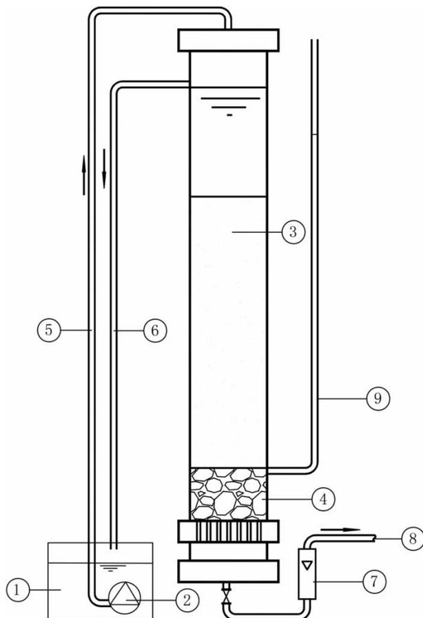
**Figure 1** | Schematic diagram of the filtration apparatus. (1) Emulsified oily wastewater tank. (2) Inflow pump. (3) Filtration column. (4) Filter supporting bed. (5) Inflow pipe. (6) Overflow pipe. (7) Flow meter. (8) Effluent. (9) Piezometric tube.
