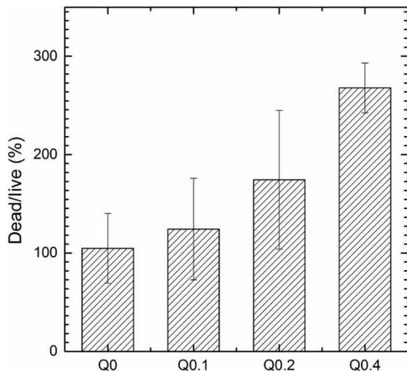
**Figure 5** | Dead/live cell ratio on sensors revealed by CLSM. The parameters were calculated from CLSM images. Error bars represent standard deviations of at least three fields of view for each surface.
